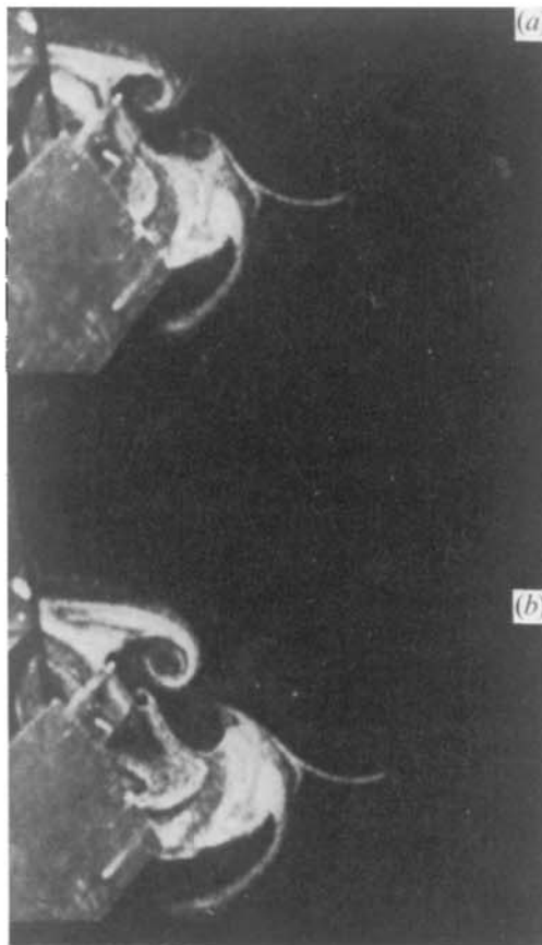
FIGURE 7. Photograph showing the breaking away from its shear layer of the first trailing-edge vortex cluster ( \alpha = 50^\circ ). (a) t = 15 . (b) t = 22 .
