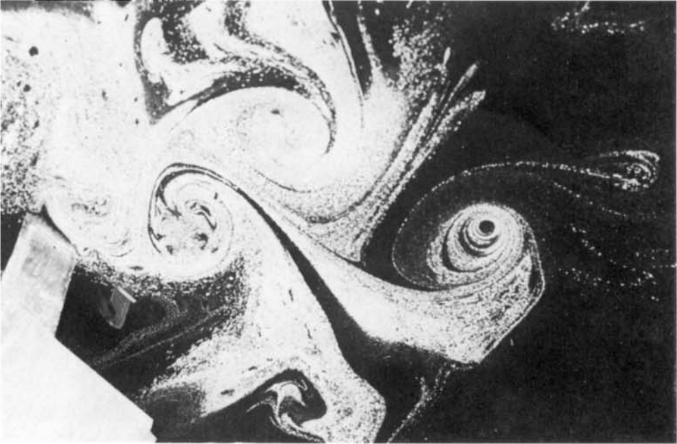
FIGURE 3. Photograph of the vortex pattern at t = 48 in the wake of a plate set at an angle of attack of 50^\circ .
