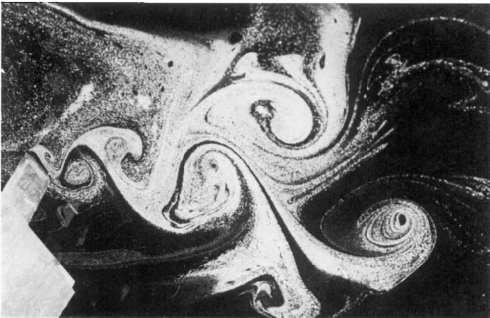
FIGURE 4. Photograph of the vortex pattern at t = 62 in the wake of a plate set at an angle of attack of 50^\circ . This should be compared with the first frame in figure 2.
