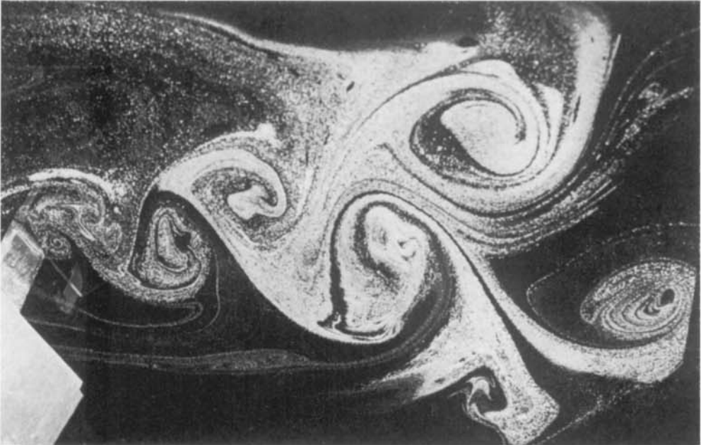
FIGURE 5. Photograph of the vortex pattern at t = 74 in the wake of a plate set at an angle of attack of 50^\circ . This should be compared with the last frame in figure 2.
